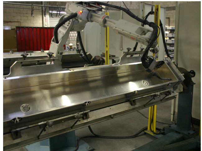
Automated Robotic Welding Process
