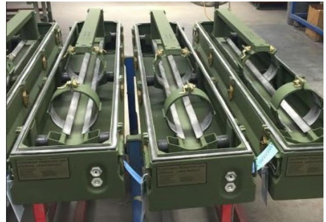
Missile Container Assemblies for Inspection
